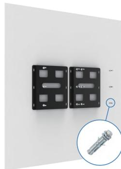
Please use **M6** expansion screws to fix the battery backsheet on the wall according to the fixed position.
