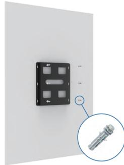
Please use **M6** expansion screws to fix the battery backsheet on the wall according to the fixed position.
